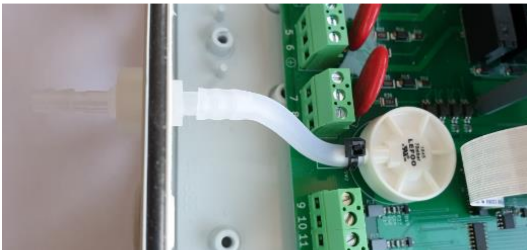
Figure 5 - Pressure switch tubing
