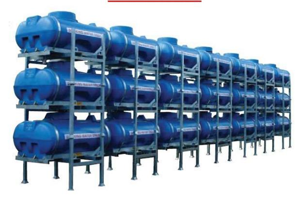
**TANK:** Polyethylene moulded tank, elliptical in section, baffled, blue approved for drinking water. Fitted with a 22" Diameter lockable outer hinged manlid cover, inner sealed vented manlid. Tank secured to frame with 2 stainless steel straps. Internal anti surge baffle. 2 rear lockable brass draw off taps.
